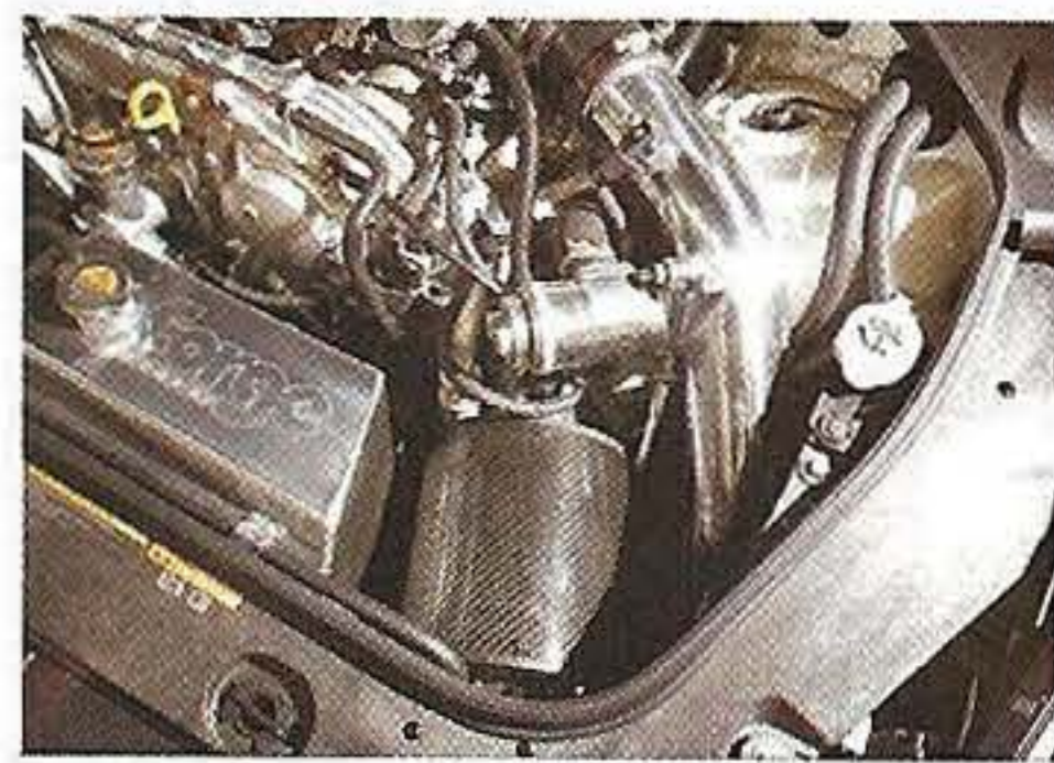
Right: new turbos help lift power by 232bhp and torque by 217lb ft; engine internals remain standard. Above: on-road driveability has been maintained. Below: body kit is by Mine's
